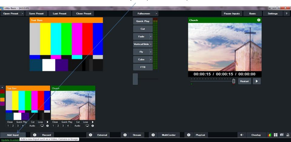
For Input Select Desktop Capture, and select the computer that you installed the software on, Press OK
